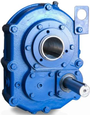
Aurora Motors speed reducers are enclosed shaft-mount-type units with double reduction ratio, either belt driven or direct coupled. Speed reducers are mounted directly on the driven shaft and utilize an adjustable torque arm to connect the gear case to the supportive structure. Our shaft mount reducers are direct replacements for popular name brands.
